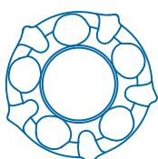
The air variator allows adjustment of jets from the nozzles using the Venturi procedure based on an intake of air into the water circuit. If you want a full-power massage, the air variator has to be unscrewed and inversely to obtain the desired massage power.
